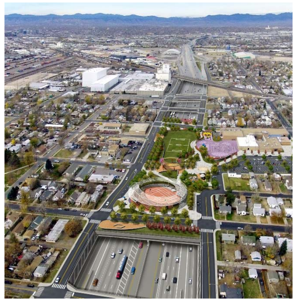
Bird's-eye view simulation of Partial Cover Lowered Alternative looking west from above Fillmore Street (Note: Preliminary design, will be revised during the public input process.)
