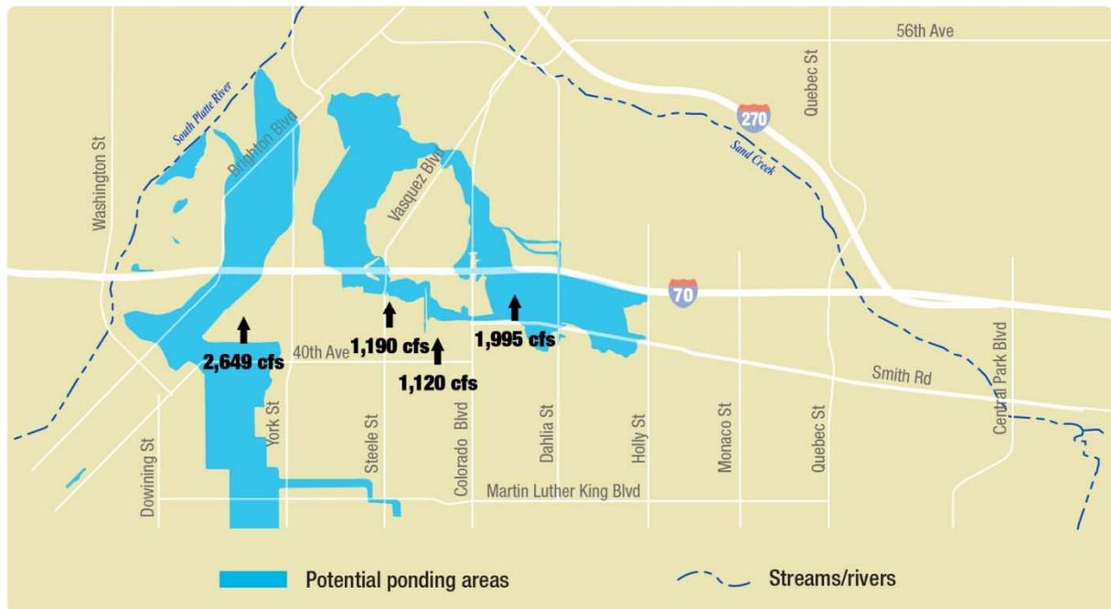
Denver's *Storm Drain Master Plan* identified substantial offsite flows through the area, including surface overflows crossing I-70 between Brighton Boulevard and York Street, near Steele Street/Vasquez Boulevard, and between Colorado Boulevard and Dahlia Street. The Denver standard is to design local storm drain systems for a 20-percent annual chance (five-year) storm event.
